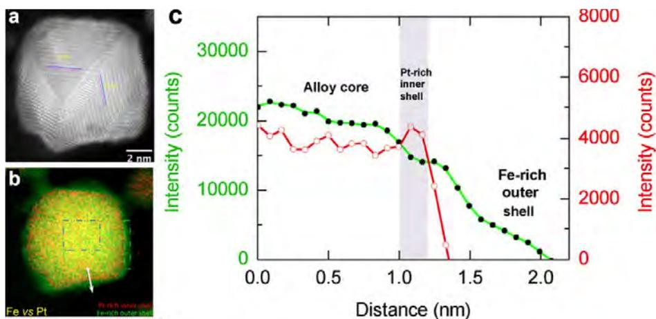
**Figure 1.** (a) and (b), STEM-HAADF and Pt versus Fe STEM-EELS composite map of a heat-treated Pt-Fe nanoparticle, respectively. (c) EELS line profiles of Fe L-edge (green) and Pt M-edge (red) taken along the white arrow highlighted in (b).
