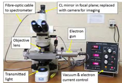
**Figure 2.** A photograph of the optical CL system at Acadia University equipped with a vacuum stage, electron gun and controller. It is presently configured for CL spectroscopy and the fibre-optic adaptor at the top can be replaced with a CCD camera for CL imaging. The instrument is a Reliotron from Relion Industries, LLC.
