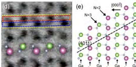
**Figure 1:** (a) HAADF image showing the oscillatory intensity at the atomic-level within the InGaN QDs, (b) integrated intensity line profile from boxed region. (c) Line profiles of the ABF image in (d), including both projected columns (Total, black line from yellow box), and separating into Top (red box) and Bottom (blue box) columns. (e) Model of ordered InGaN from the preferential incorporation of In at the reduced N-coordination site ( $N=2$ ).
