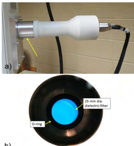
**Figure 5.** a) A side view of the optical filter holder showing its mounting location between the spectrometer casing and the PMT; b) A view of the top of the filter holder highlighting the red-block dielectric filter and supporting o-ring.
