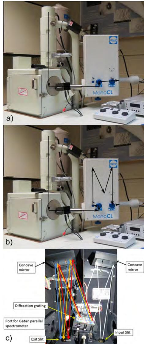
**Figure 4.** Light paths in a Gatan MonoCL3 CL system for: a) panchromatic imaging; b) monochromatic imaging and spectroscopy; and c) from the rear of the spectrometer where the components are displayed.
