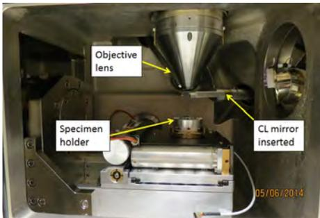
**Figure 3.** A photograph of the inside of the specimen chamber of a JEOL LV5900 SEM displaying the location of the light collection mirror of a Gatan MonoCL3 CL system.
