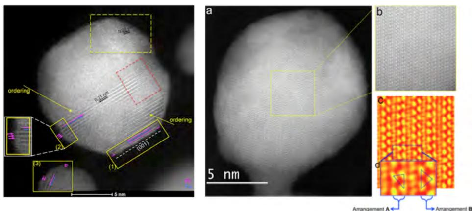
**Figure 2.** , STEM-HAADF image of an ordered PtFe particle illustrating Pt atoms wedged at the surface (highlighted in the yellow boxes).
