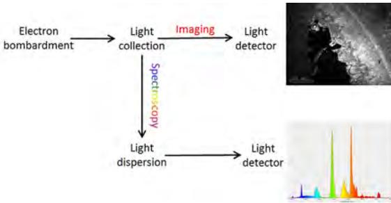
**Figure 1.** A simplified schematic diagram of the typical CL system flow from electron bombardment to light detection and spectroscopy. The panchromatic CL image is from a brachiopod sample and the spectrum was collected from the light emitted from a fluorescent bulb.
